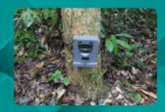
TEREA provides a fleet of high-quality camera traps resistant to the challenging conditions of deployment in humid equatorial forests in Central Africa.
